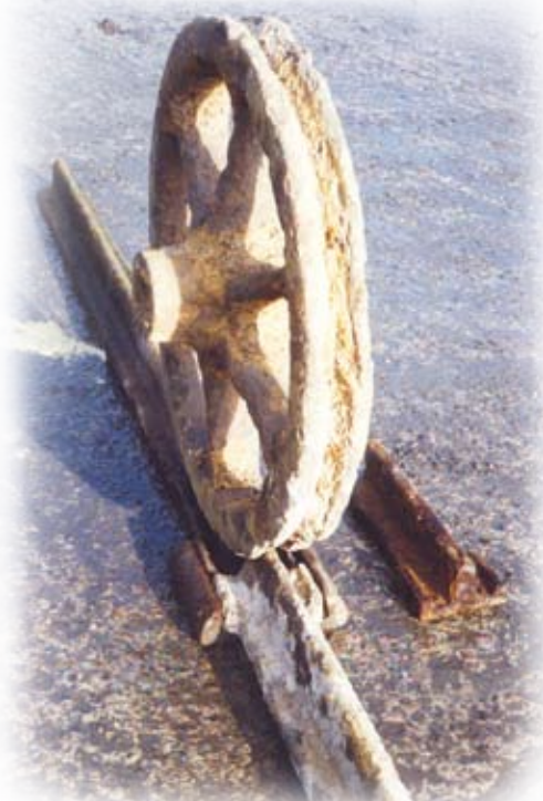
The original rails were cast iron with a cross section of an upside-down T – they had a tendency to break near the join. The truck wheels had a flange on each side.
